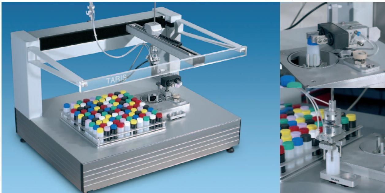
Taris is a low cost system for taring and weighing of vials with the option of decapping and capping. The system is designed for batches of 100 to 200 vials per loading. The processing time is about 1 minute per vial (including screwing the caps off and on again). The system can run completely unattended. It produces a file with the weights and a log file of the complete run. An optional barcode reader can check the barcode while the vials are decapped and capped.
